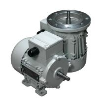
Anaheim Automation's AC Industrial Motors come in two different mounting options: Leg (foot) mount and the flange mount option. Both the ACI-PMCB040-4R4LAT and the ACI-PMCB040-4R4FAT run up to 1730 RPM and deliver 400 Watts of power. All of our ACI PMCB040 AC Industrial motors are 3 phase, and can be wired to run off of 220 VAC or 380 VAC at a frequency of 60 Hz.
